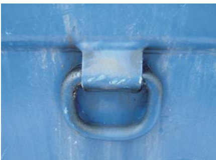
Example of a swivel type tie down point.
