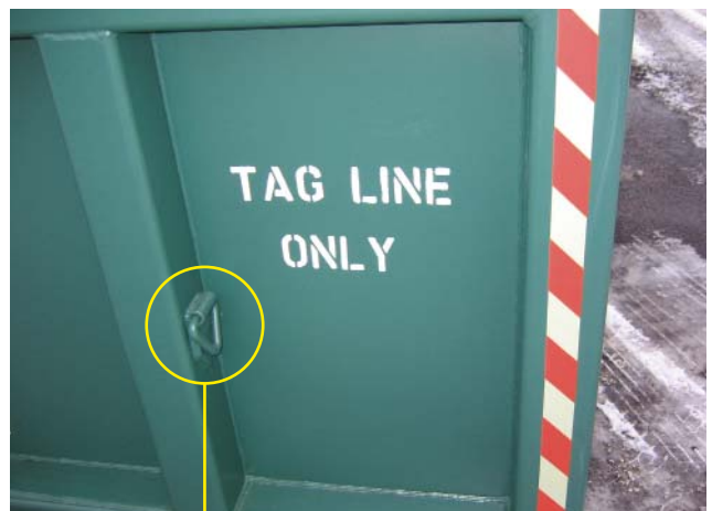
Example of Swivel Type Tag Line Fixture Point
