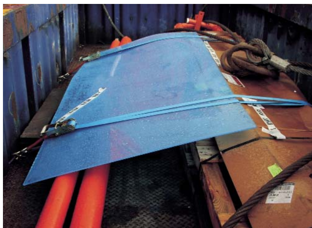
Example of partially secured backload.
