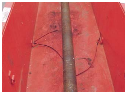
Example of poor cargo securing.
