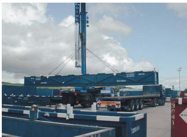
Typical lift showing a balanced load.
