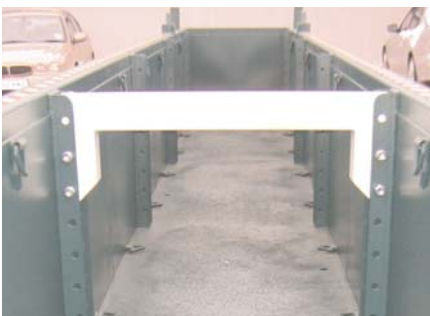
Example of a swivel type tie down point.
