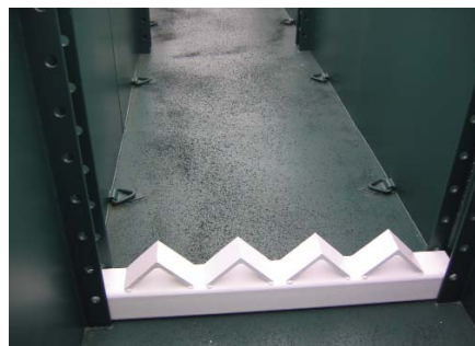
Examples of alternative restraining devices fitted to cargo baskets.
