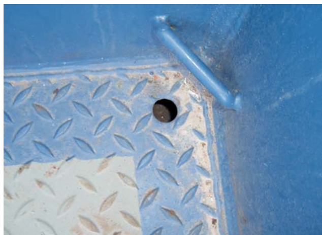
Floor of basket showing typical drainage hole.
