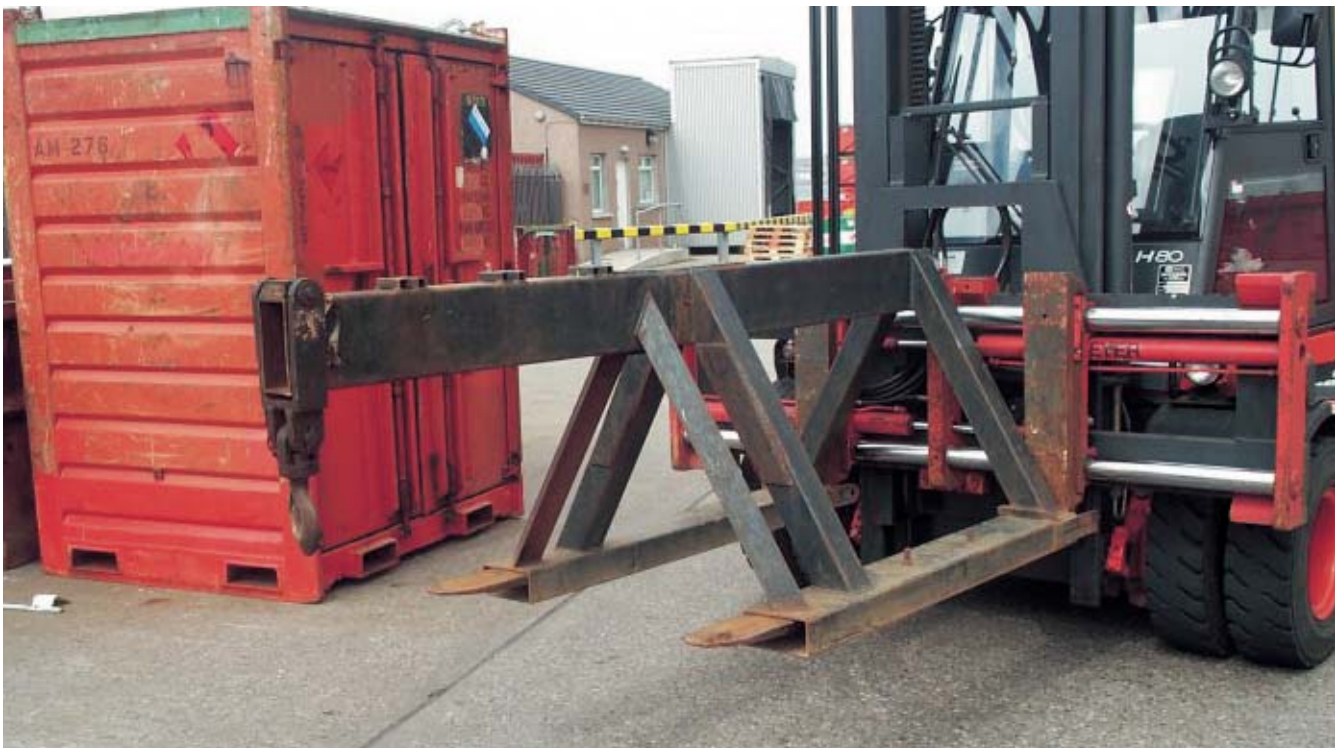
A means of lifting a basket to check for balance.
