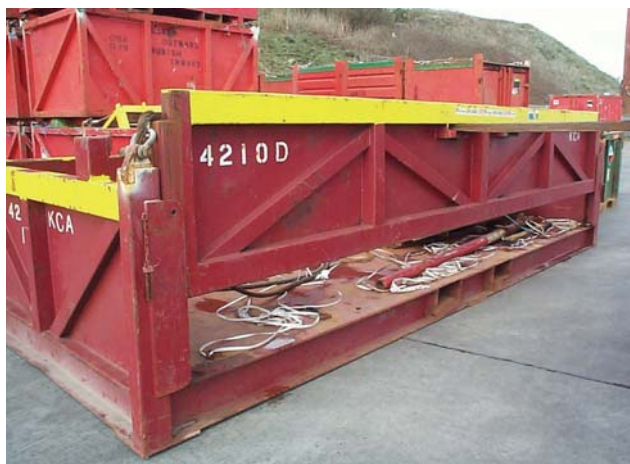
Example of where kick plate should be fitted.
