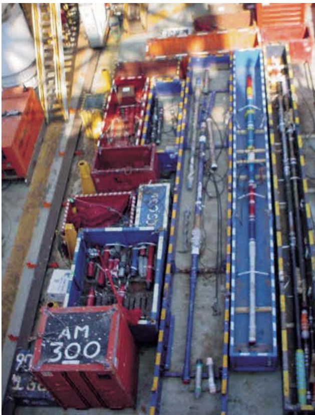
Prearranged deck cargo to accommodate cargo baskets.
