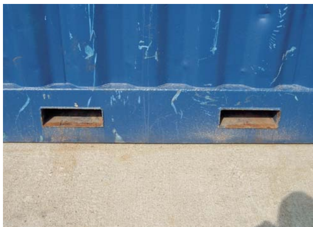
Typical Forklift Pockets.
