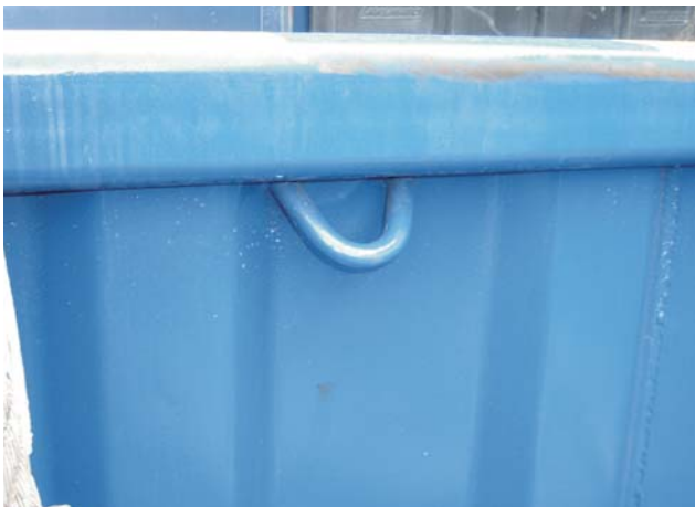
Possible internal snagging hazard.
