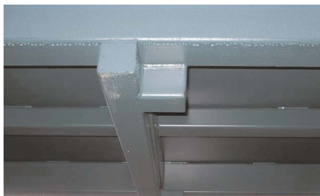
Underside view of basket stacking mechanism.
